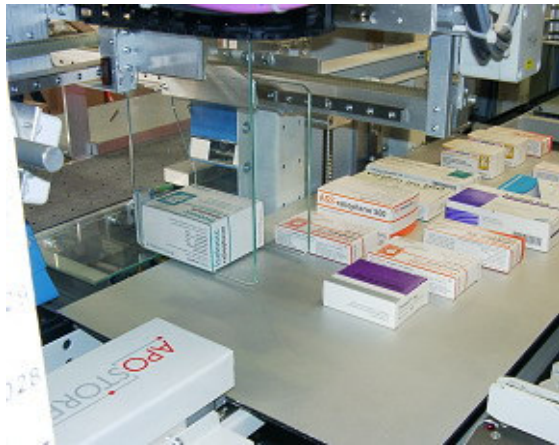
Double deep storage at intake tray
